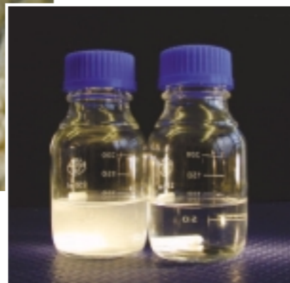
Struvite (Magnesium-Ammonium-Phosphate) in combination with sludge/polymer deposits.
