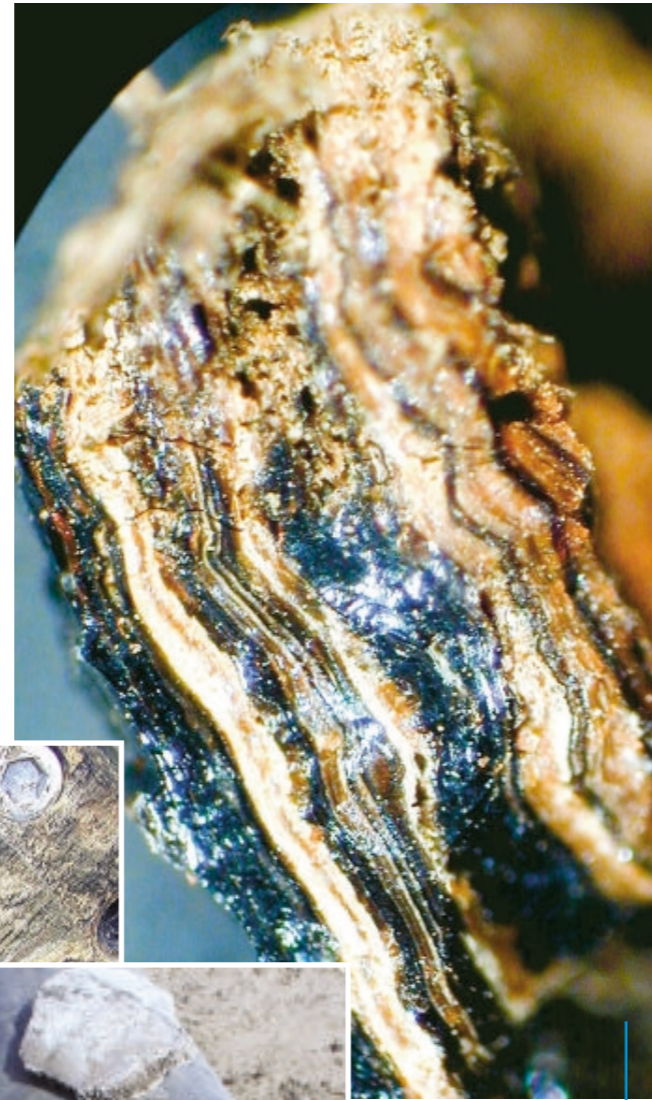
Microscope view of crystals layers (Struvite) [Mg(NH_4)(PO_4) \cdot 6H_2O]
